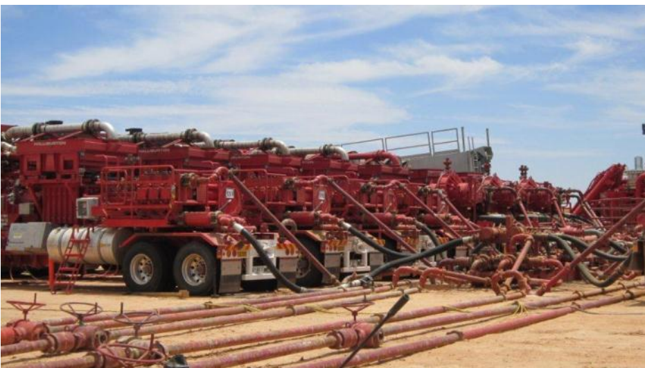
Halifax-1 hydraulic stimulation, ATP 855P, Cooper Basin, Queensland
