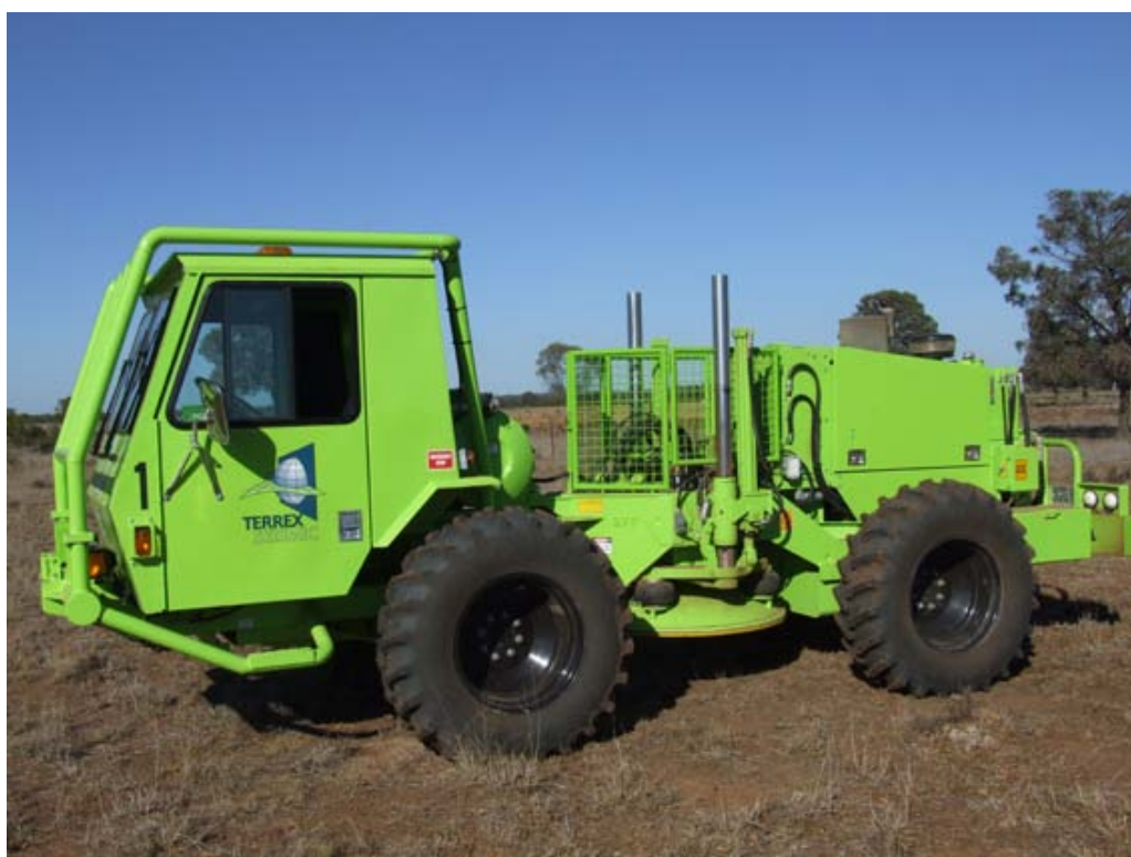
Figure 1: One of three Terrex "Eco-Vibe" trucks used in Icon's Seismic program October 2009
